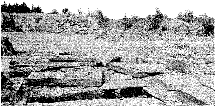
Figure 61 Three views in the quarries at Reidsville, showing the heavy sandstone beds of the Hamilton and flagstones that have been taken out. (Photographs by W. Goldring)
